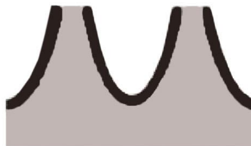
Quenching of Tooth Surface and Dedendum
